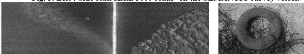
Fig 7. Example of high resolution acoustic picture by Klein 3900. Left : Tire on ripple sand (photo on Fig. 8). Right : posidonia meadow.
