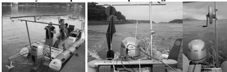
Fig. 5. Left : Side scan Klein 5000 sonar on the SEMANTIC survey vessel.
