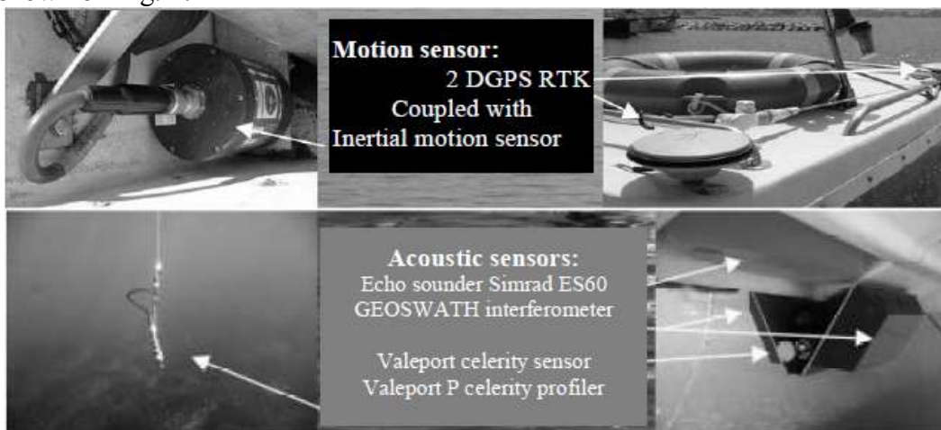
Fig. 2. Instrumentation systems. D-GPS differential RTK Leica GX1230 centimetric system - Motion sensor Coda Octopus FS185+
