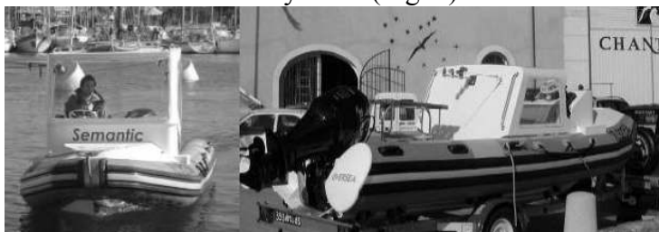
Fig. 1. Survey unit SEMANTIC : semi-rigid with removable cabin.
